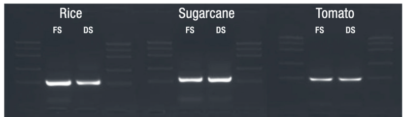
Fig 5. Comparison of fresh and dried leaf samples Amplification of 0.5 kb fragments directly from fresh (FS) and dried (DS) leaf punches (1.2 mm diameter) from rice, sugarcane and tomato. The dried samples were pretreated by addition to 100 µL of extraction buffer (1.25 w/v SDS) and incubation at 95°C for 5 minutes. 1 µL of this extract or the fresh leaf punch was used in a 50 µL PCR reaction setup using the MyTaq Plant-PCR Kit. The results illustrate that MyTaq Plant-PCR exhibits similar results from both the fresh and dried leaf samples. MW marker EasyLadder I.
